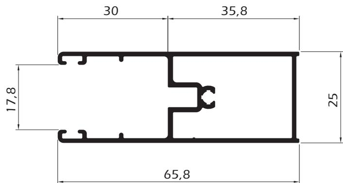
**P 1462\*** | 0,514 Kg/m | Tubo Octogonal Integrada TI-028
