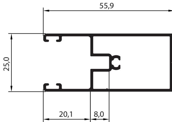
**P 1461\*** | 0,698 Kg/m | Guia Lateral Integrada TI-019
