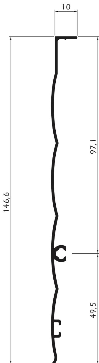
**P 1429\*** | 0,836 Kg/m | Tampa Interna Integrada TI-006
